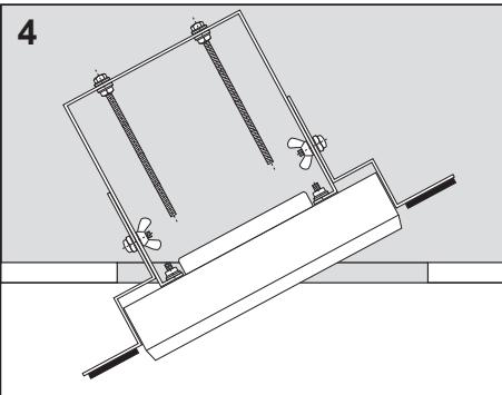
Remove ceiling plate, reflector, washered mounting nuts and downlight body from plaster assembly.
